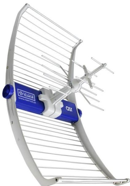
Modern broadband asr classic antenna is dedicated to reception of DVB-T digital-TV signals. It has a large energy gain and a built-in ultra low noise pre-amplifier that can be powered with voltage ranging from 5 to 24V. Low level of own noise of first amplification level is significant to obtain a good signal quality (high S/N ratio).
